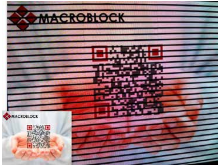
Figure 46. “the traditional switch-type” Drivers – high grey scale/low-refresh impact on Two-dimensional Code Recognition (distortion)
