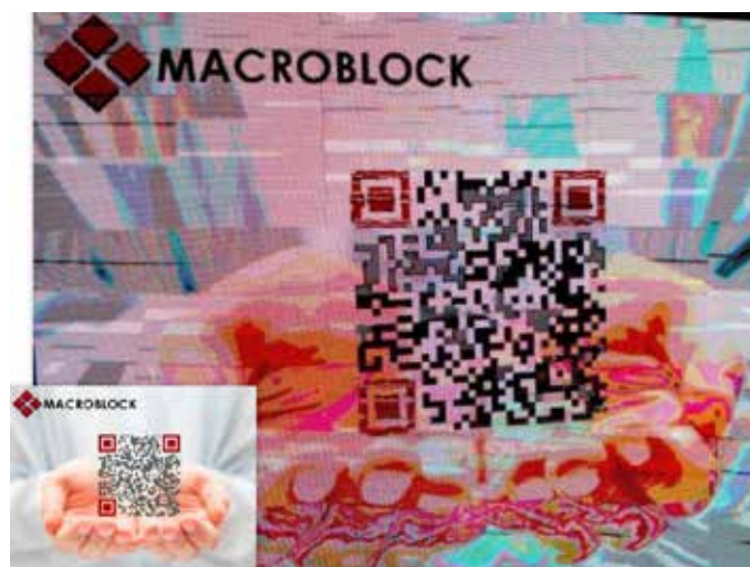
Figure 45, “traditional switch-type” drivers – high refresh/low grey scale impact on Two-dimensional Code Recognition (Blending)
